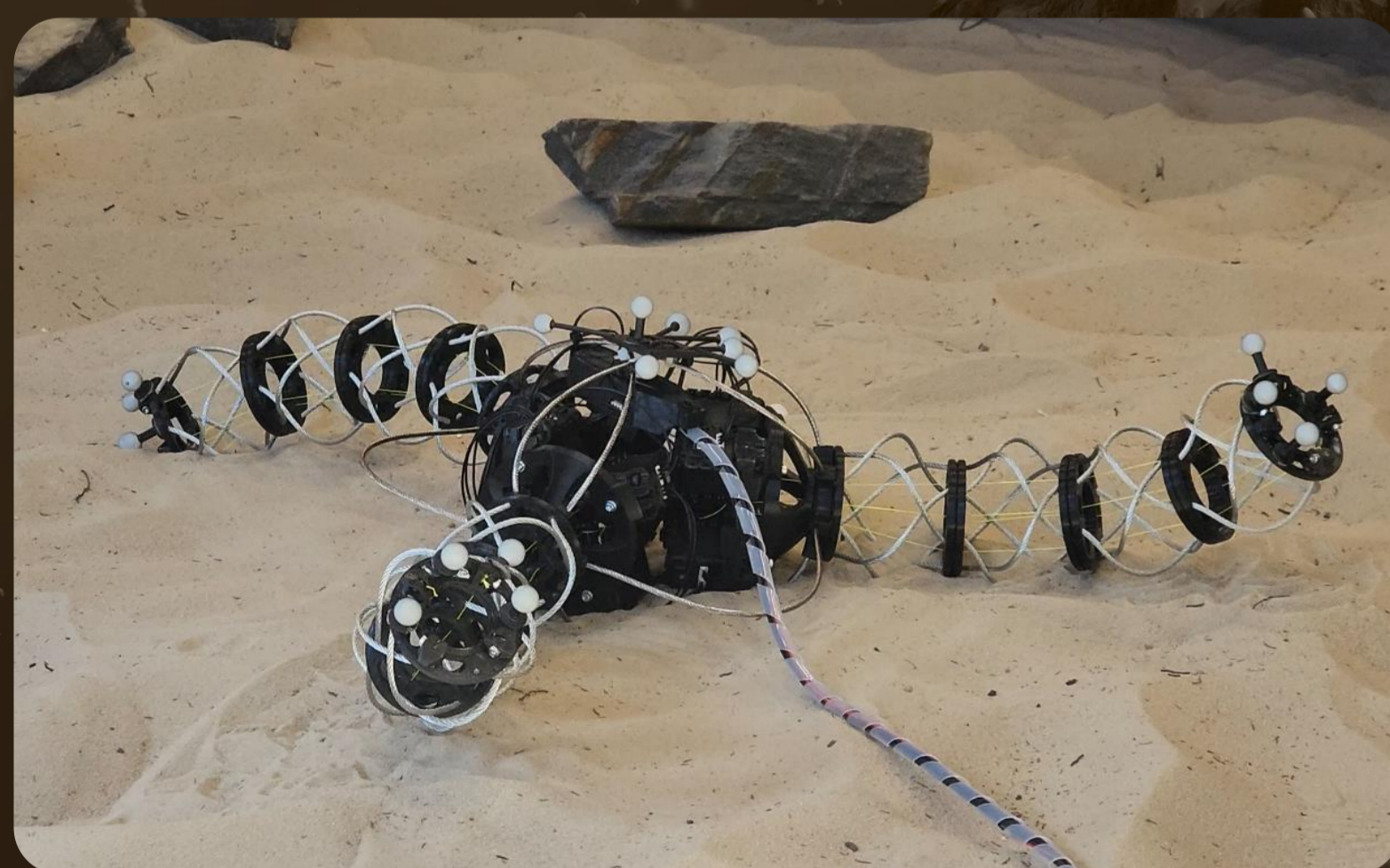
A soft robotic tripod undergoing locomotion testing in sand, above and Space Resource Technologies LHS-1E lunar regolith simulant, below.
