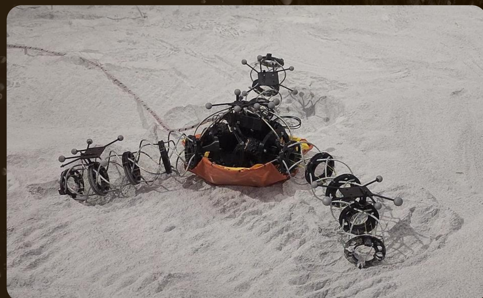
A soft robotic tripod undergoing locomotion testing in sand, above and Space Resource Technologies LHS-1E lunar regolith simulant, below.
